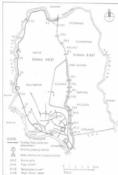
Figure 1: Existing flood control and drainage infrastructures during 1998 flood.
