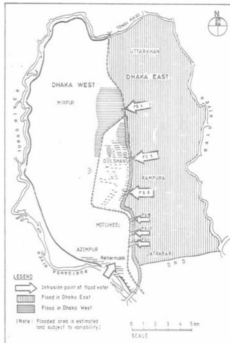
Figure 2: Areas flooded by river water and floodwater intrusion points during 1998 flood.
