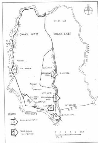
Figure 4: Locations of pumped drainage in Dhaka West during 1998 flood.
